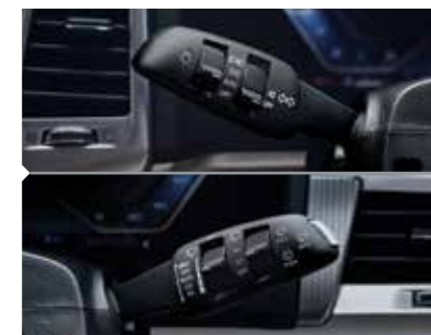
Headlamp control and automatic washer switches
