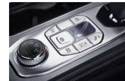
Electronic parking brake with auto-hold function
