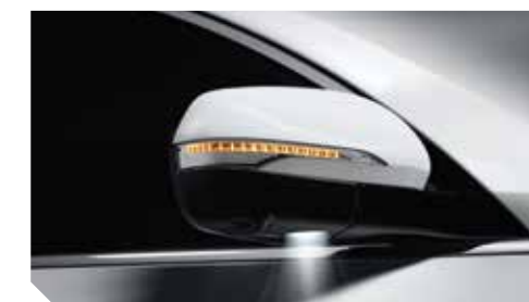
Side repeater and puddle lamp mounted on the back of the outside mirror
