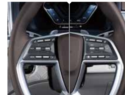
Remote control switches and cruise control system on the steering wheel
