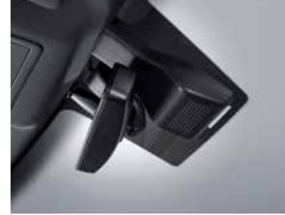
Rain-sensing and automatic light control unit (SPR only)
