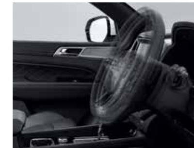
Tilt and telescopic steering wheel system
