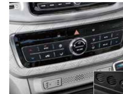
Dual-zone fully automatic air-conditioner; 3rd row air conditioner (SPR only)
